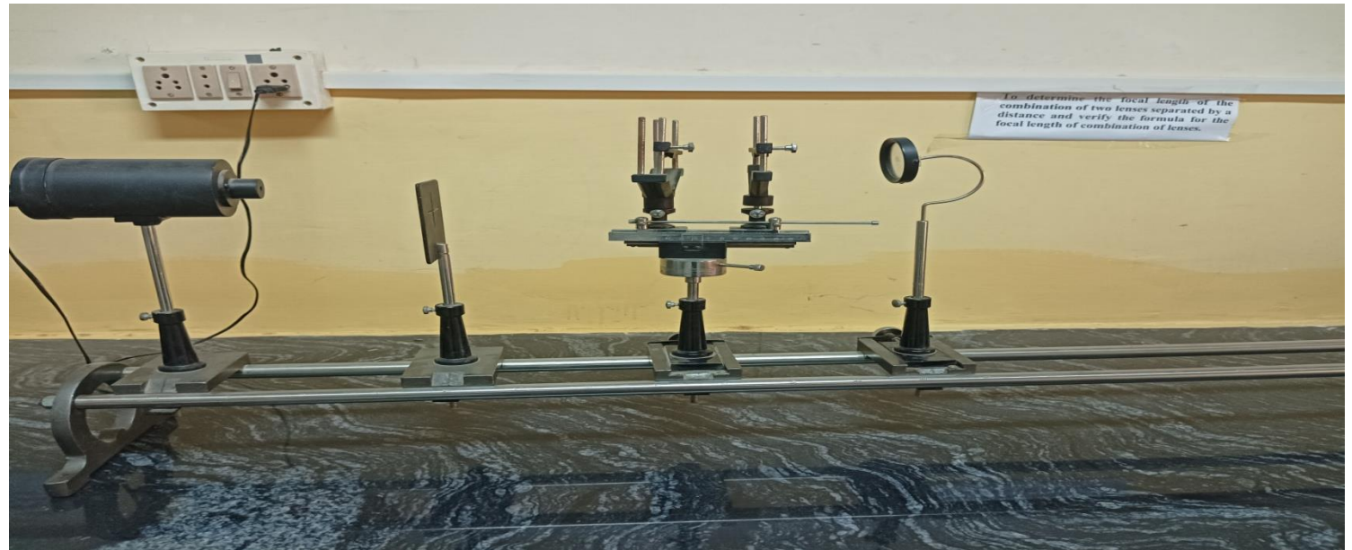
Focal length of two lenses by Nodal slide
